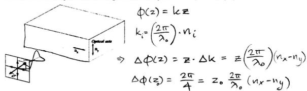
(b) Assume the crystal thickness is a quarter wave plate for a free-space  $\lambda_0$ , shifting the x- and y-components by 90 degrees. Write an expression for the electric field after the light exits the crystal. Assume that  $n_x > n_y$  in the crystal. [10]
