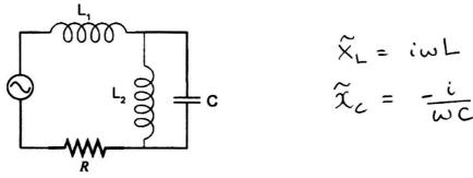
(a) What is the circuit's total impedance, magnitude and phase angle? [8 points]
