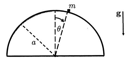
[20 points] A particle of mass m slides down a frictionless hemispherical cap (of radius a) in a uniform gravitational field with acceleration due to gravity g. See the figure.
