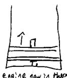
eagine now in thermal contact with the heat meruoir at Ti. Engine absorbs hart q, from reservoir
