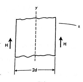
where we have used the identity curl curl = grad div  $-\nabla^2$ . A solution must be found obeying the boundary condition  $\mathbf{B}(\pm d) = \mathbf{H}_0$ . The solution desired is
