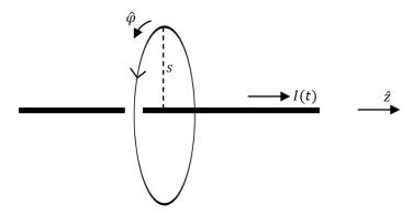
By the azimuthal symmetry of the setup, the magnetic field of a single wire points in the  $\hat{\varphi}$  direction and depends only on the distance to the wire s:  $\mathbf{B}_1 = B_1(s,t)\hat{\varphi}$ . Applying the integral version of Ampere's law, we get
