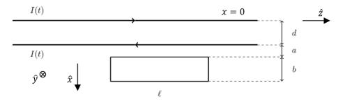
By the right-hand rule, the direction of the magnetic fields in the area of the loop can be determined (assuming I(t) > 0): The magnetic field due to the top wire points in the  $+\hat{\mathbf{y}}$
